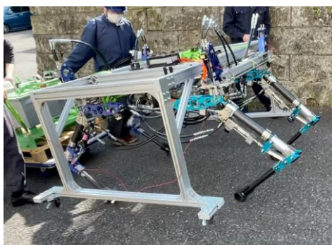
Figure4-11 Walking experiment on Quadruped outdoor field robot
