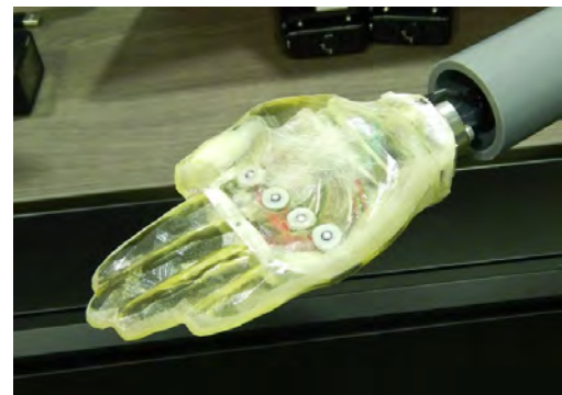
Figure 4-8 Hand for a New Underwater Humanoid Robot
