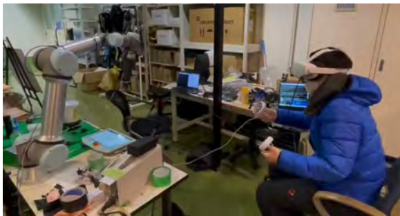
Figure 4-10 Experiment of VR Remote-Controlled Robot Operation
