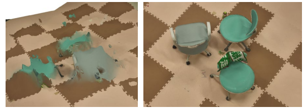
Figure 4-7 Reconstructed 3D model (left: without camera control, right: with camera control)
