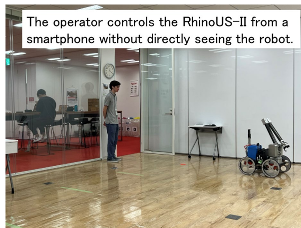
Figure 4-13 Teleoperation experiment from a smartphone
