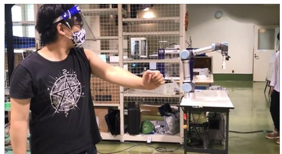
**Figure4-9 Working remotely with a high-speed motion capture system for control**
