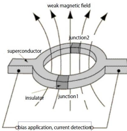
**Figure4-16 Schematic drawing of a Superconducting Quantum Interference Device (SQUID)**
