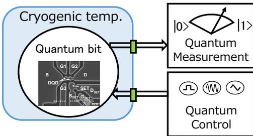
Figure4-13 Schematic image of quantum bit measurement system
