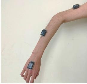
**Figure4-7 Inertial sensor attached to the human body arm**
