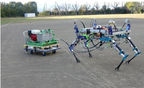
**Figure4-11 Quadruped outdoor field robot**
