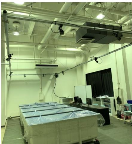
**Figure4-8 Ceiling-mounted optical cameras of motion capture system**
